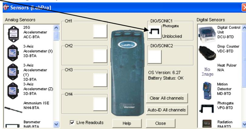
Right click on the picture of the photogate and a set-up menu will come up telling the computer how you want to use the photogate. We want to measure the change in time for several blockings of the picket fence so we can see how the velocity changes as the fence fall through the photogate- that is the *Motion Timing* function, so be sure it is checked.
