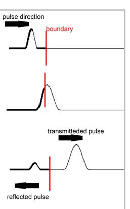
less amplitude in reflected pulse
