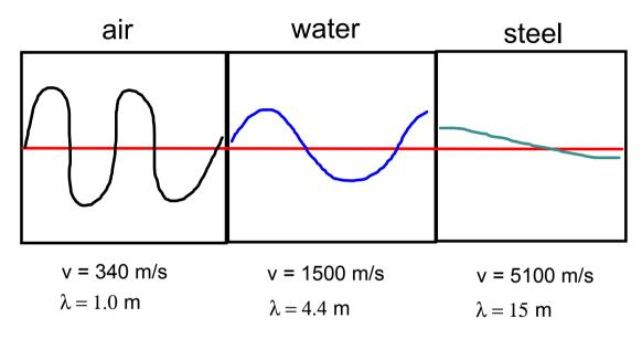
Note: 1) The wavelength is shortest in air and longest in steel! (shorter  $\lambda$  in air because slower velocity)
